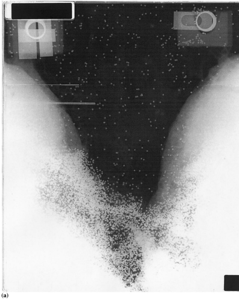
Fig. 5. Radiographs for runs ZCN. These are repeat runs and the five images (a)–(e) were obtained at times 0.2, 0.25, 0.3, 0.35 and 0.4 s following initial contact of the cloud with the water.
